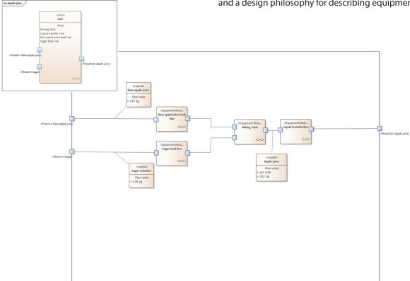
With the new solution, units can be assembled into devices and connections can be defined and detailed by physical units (e.g. liquid, gas, etc.).
