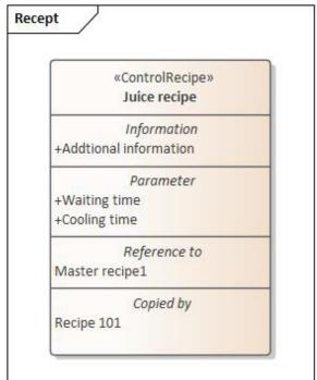
Procedure including material flow can be defined at different levels (e.g. Procedure, Operation, Phase and Action). Recipes as the basis be defined including parameters and additional information.
